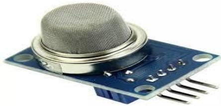
Fig 4: MQ2 Gas Sensor
