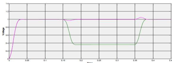
Figure.4.Source and load rms voltages during sag
