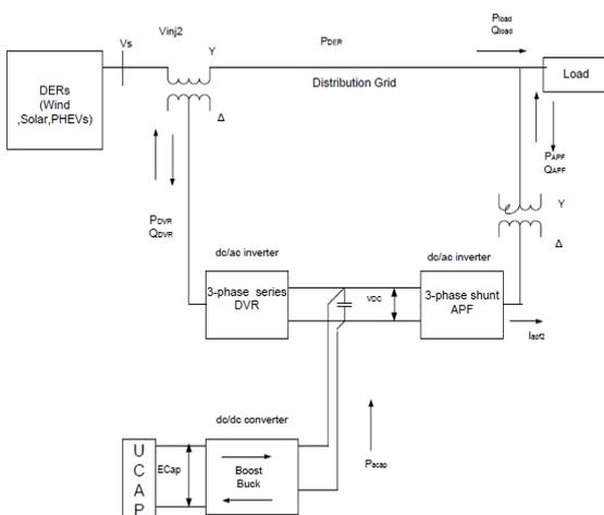
Figure 2. Block diagram of the Power Conditioner with UCAP Energy Storage
