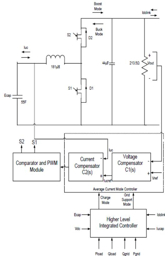
Figure 3. Model of the bi-directional dc-dc converter and its controller
