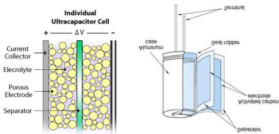
Figure 1. Individual capacitor cell
