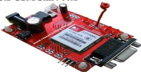
Figure.2-GSM Sim 900A
