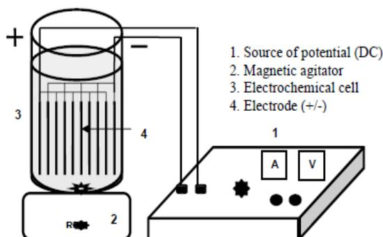
Fig. No 2 Typical Electrocoagulation system
