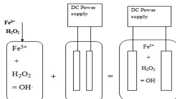
Fig. 2 Electrochemical Process
