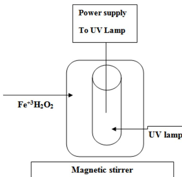
**Fig.1 Photo Fenton process shows in the schematic diagram**
