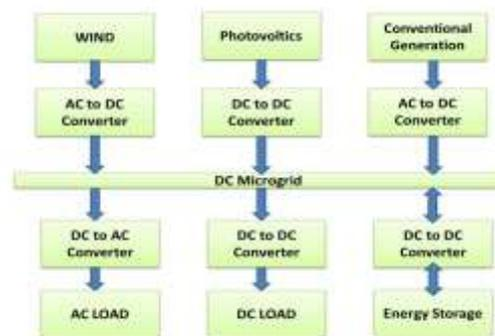
**Fig No .2 Block diagram of Microgrid power system**
