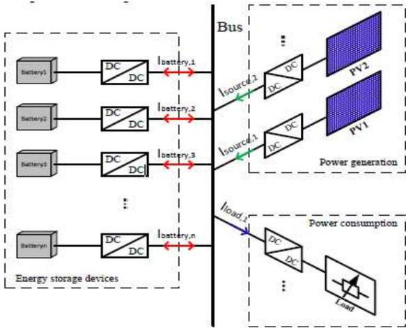
**Fig. No 3. Configuration of a typical DC Micro grid**
